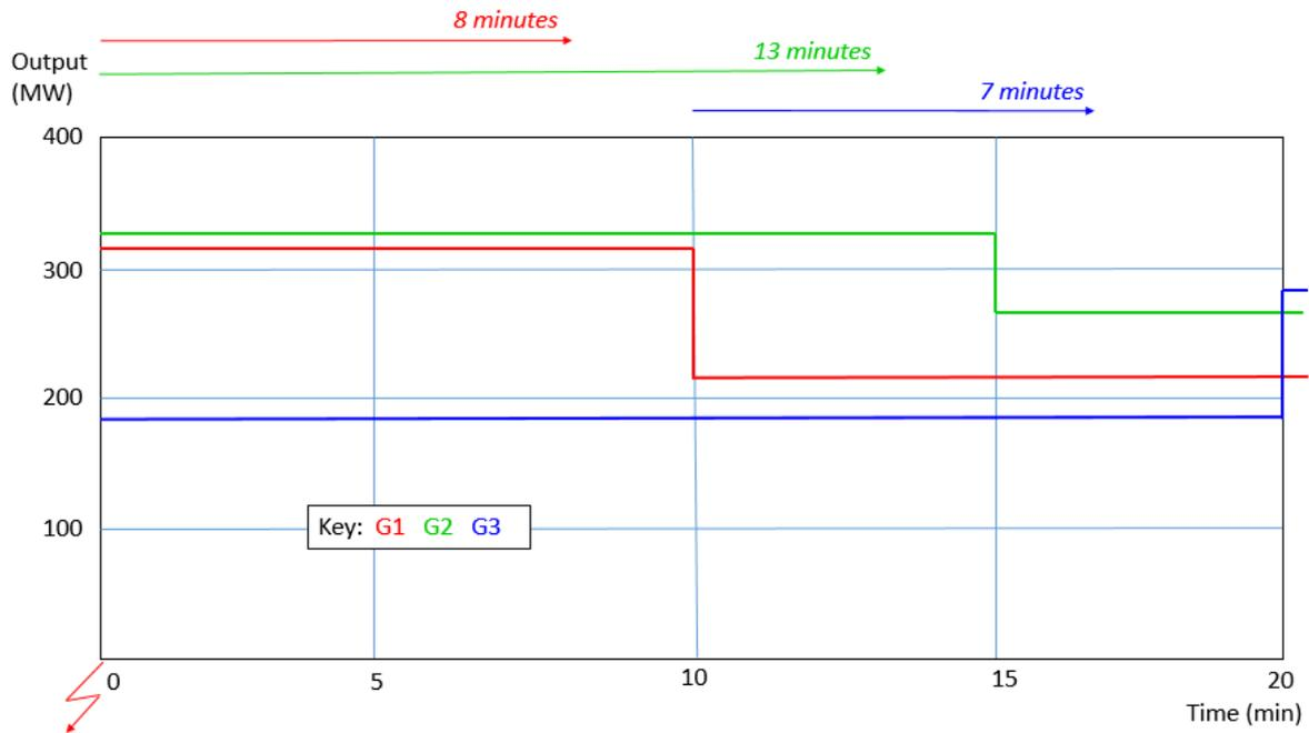
Figure 26.11.1: RAS timings in Multiple Time Phase Contingency Analysis
